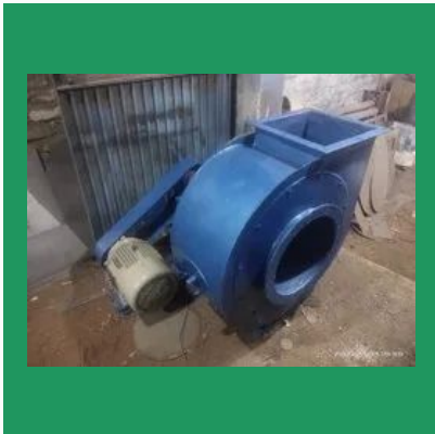
Industrial Air Blower
